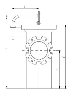
Up to 16 Bar G **Design Pressure:** 3mm **Corrosion Allowance:** ANSI B16.5 150/300RF Flanges: ASME sec. V Ⅲ. Div.1 **Design Code:** 15, 30 Bar G **Test Pressure: Typical materials of construction:** (or equivalent, depending on availability) **Body and Cover:** ASTM A516-70 **ASTM A105** Flanges: **ASTM A106** Pipe: **Stainless steel Basket & screen:** A240-304/316/316L
